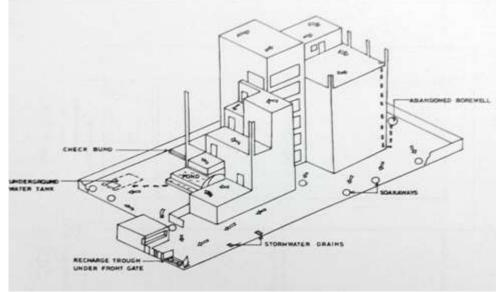
Fig-1: Water Harvesting System in Building
