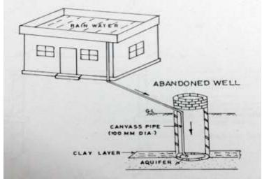
Fig-2: Schematic Representation Of Water Collection
